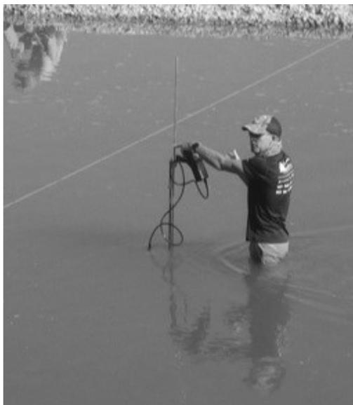
As seen in the photo, a calibrated wire called a tag line is stretched across the river or stream. The hydrologist then measures the depth of the water along selected points (generally 25 cross sections) on the tag line, then multiplies this depth by the width of the segment to get the area. Then, the velocity of the water is measured at a point a little more than one-half the depth.
